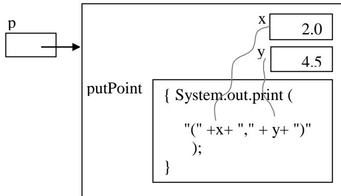
*Every object we create has a copy of each instance method in the class.* In contrast, only one copy of a static method exists, and it exists from the time the class is loaded at run time. So every `Point` object has a version of `putPoint`. To emphasise that we really do get a copy of `putPoint` inside each `Point` object, suppose we created two `Point` objects:
