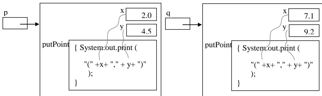
Observe that each copy of `putPoint` differs slightly from the others in that each mention of `x` and `y` in the body of `putPoint` is locked onto the `x` and the `y` in the object where the copy lives. This is indicated by the wavy lines in the diagram above.
